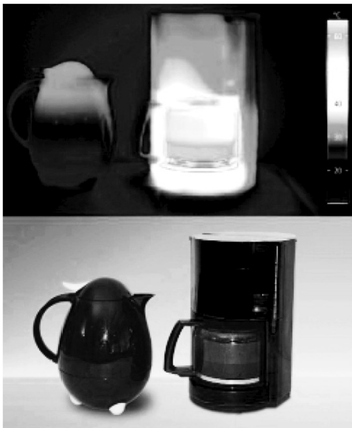
Figure 36: Comparing a Passive House building to a conventional building is analogous to comparing an insulated thermos (left) to a coffee carafe on an active burner (right). Through continuous insulation and air tightness the thermos passively conserves the coffee's heat whereas the open carafe requires active heating to keep the coffee hot. The infrared image (at top) shows the stark difference in heat loss between the two containers. The concept applies the same for conserving air-conditioned cooling as well (Source: Passivhaus Institut).
